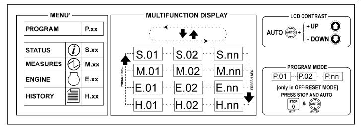
This area, which is composed by a display and the buttons, allows the visualization of the configuration parameters, the plant status, the electrical measures, the engine analogue and digital measures, the digital IN/OUT signals acquired and the historic visualization of the events and the measures.
