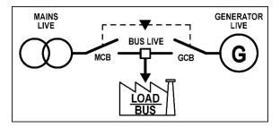
measures to determine when the **Mains** is back. When the **Mains** is back, the device command the **MCB** and **GCB** circuit breakers to supply the **Loads** by the **Mains**.
